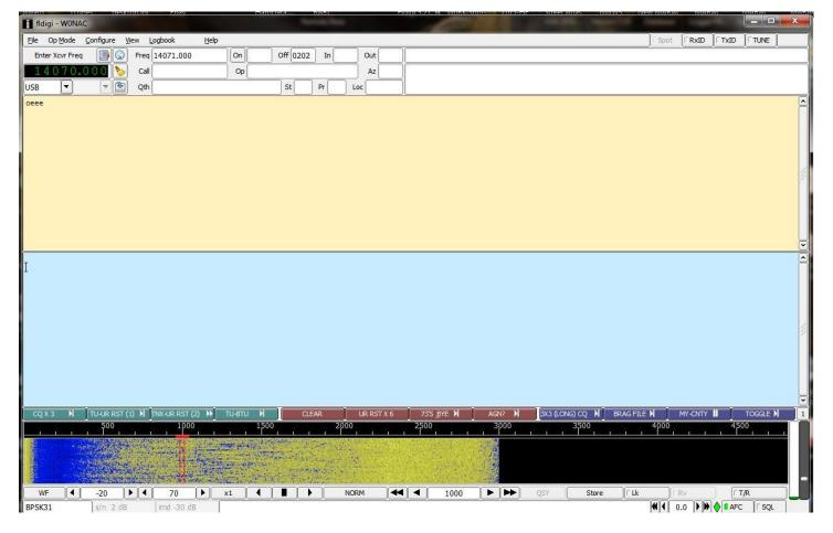
Note that the SQL (squelch) control at the lower right is OFF and AFC is ON.
